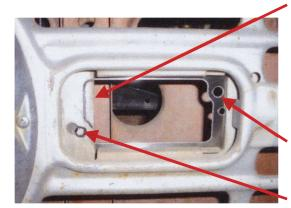
You will solve the first problem by removing material with a file or dremel tool. Mark the area to be removed and then use your choice of tool to remove the material. Temporarily holding the adapter plate in place may help you see what needs to be relieved. You can also keep trying to fit the new signal in and see where it's hitting.
