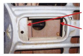
If you try to fit the early turn signal into this Opening, it won't fit because of interference here.
