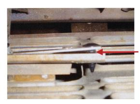
Now go ahead and put the adapter plate in place behind the grille. The turn signal will hold it in place once the installation is done, but a plastic ratchet fastener has been provided to hold it in place if you care to use it. This picture shows the plastic fastener only pushed part way in.
