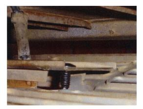
The plastic fastener is now fully installed and you are ready to mount the new turn signal.
