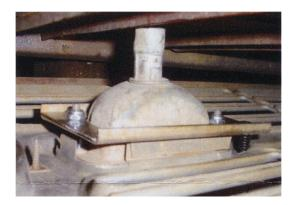
Use the nuts that are supplied with the adapter to mount your early turn signals. The nuts will not ping up against solid metal so don't let yourself over tighten them. When the turn signal gets snug stop tightening the nuts.
